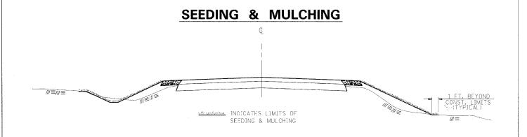
IN GENERAL, ALL EARTH SURFACES DISTURBED DURING CON-STRUCTION OPERATIONS SHALL BE SEEDED AND MULCHED UPON COMPLETION OF ALL GRADING OPERATIONS.
