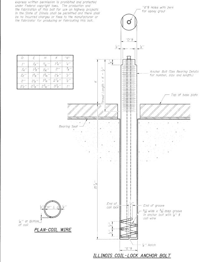
The Illinois Coil-Lock Anchor Bolt is a proprietary
