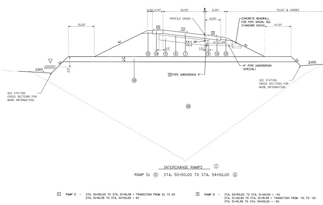
RAMP D - STA. 50+50.00 TO STA. 51+91.99 = TRANSITION FROM -3.33% TO -2%
