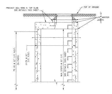
SECTION "A-A" STANDARD MANHOLE BARREL
