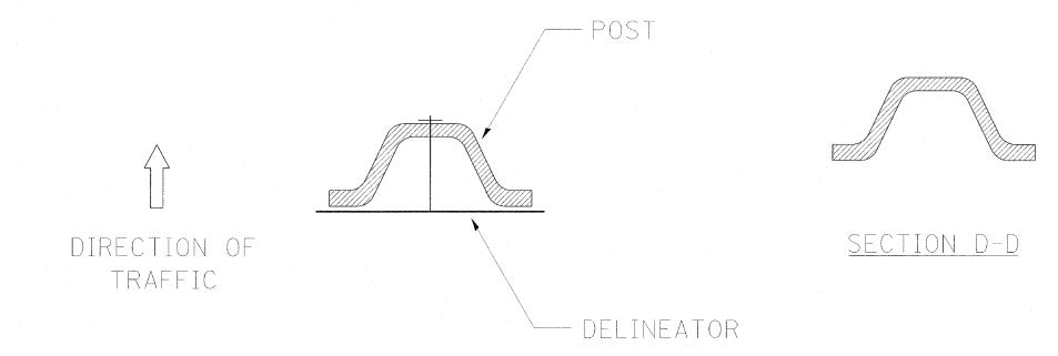
DELINEATORS SHALL BE INSTALLED ACCORDING TO STANDARD 635001 EXCEPT THAT THE POST SHALL BE ROTATED 180°. THE POST WILL HAVE THE WIDE SIDE FACING TRAFFIC AND THE DELINEATOR ATTACHECD AS SHOWN ABOVE.
