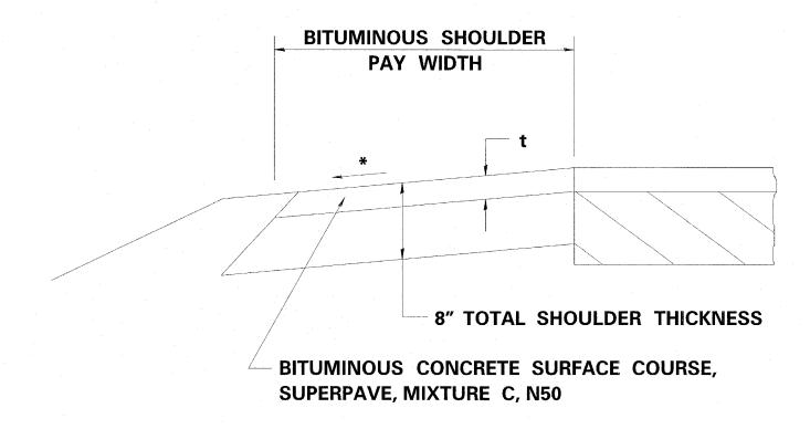
t = SEE TYPICAL SECTIONS FOR THICKNESS
