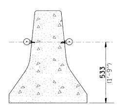
REFLECTOR MOUNTED ON CONCRETE BARRIER
