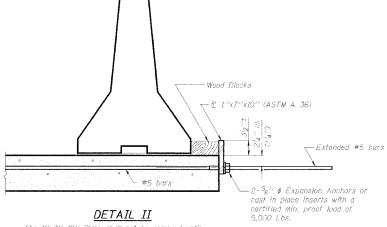
The I"x7"x10" Plate shall not be removed until Stage II Construction forms and all reinforcement bars are in place and the concrete is ready to be
