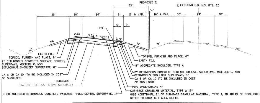
WESTBOUND U.S. ROUTE 20 LOCATION SUPERELEVATION 'a' STATION 1771+68.00 TO STATION 1798+77.00 5.3% S.E. 1:6 1:6 2' & VAR. STATION 1854+51.00 TO STATION 1857+00.00 5.3% S.E. 1:4 1:4 & FLATTER 4' 1:6 2' & VAR. STATION 1857+00.00 TO STATION 1886+00.00 5.3% S.E. 1:4 1:4 & FLATTER STATION 1886+00.00 TO STATION 1903+13.00 5.3% S.E.
