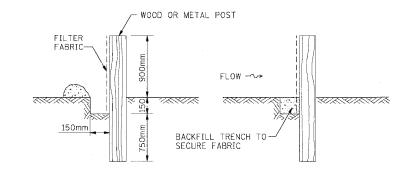
SILT FILTER FENCE DITCH CHECK
