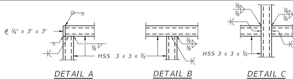
All steel rail elements shall be galvanized according to the Special Provision for Handrails and Railing and Article 509.05 of the Standard Specifications.
