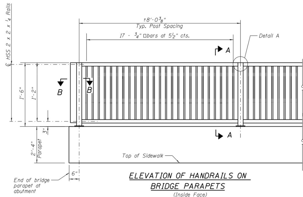
**ELEVATION OF HANDRAILS ON BRIDGE PARAPETS**
