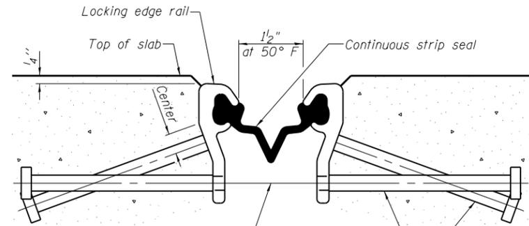
7/16"  $\phi$  holes at 4'-0" cts. for 3/8"  $\phi$  bolts. All bolts shall be burned, sawed, or chipped off flush with the plates after forms are removed, typ.
