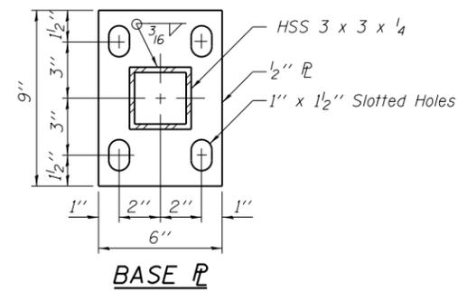
All steel rail elements shall be galvanized according to the Special Provision for Handrail and Railing and Article 509.05 of the Standard Specifications.
