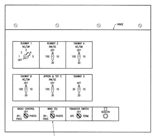
WIND TEE NO LONGER EXISTS. REPLACE WIND TEE CONTROL SWITCH WITH TAXI GUIDANCE SIGN CONTROL SWITCH: "ON-OFF" 2-POSITION SWITCH, AS DETAILED. INCLUDE UPDATED LEGEND PLATE LABELED "TAXI SIGNS" WITH "OFF" & "ON" POSITIONS IDENTIFIED.
