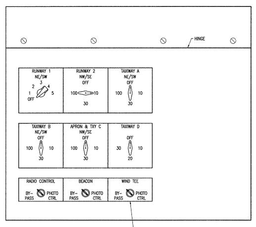
WIND TEE NO LONGER EXISTS. REPLACE WIND TEE CONTROL SWITCH WITH TAXI GUIDANCE SIGN CONTROL. SWITCH: "ON-OFF" 2-POSITION SWITCH, AS DETAILED. INCLUDE UPDATED LEGEND PLATE LABELED "TAXI SIGNS" WITH "OFF" & "ON" POSITIONS IDENTIFIED.
