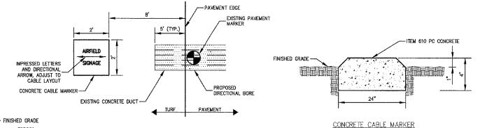
RESTORATION PER SPECIF. SECT. 108-3.5 CABLE IN UNIT DUCT (+)(+) 1'--0" MAX.
