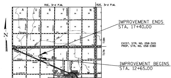
IMPROVEMENT CONSISTS OF THE REMOVAL OF A SINGLE SPAN CONCRETE DECK ON WF BEAM IMPROVEMENT CONSISTS OF THE REMOVAL OF A SINGLE SPAN CONCRETE WINGWALLS, O-O DECK = 19'-6", BK.-BK. ABUTMENTS = 27'-0" AND THE CONSTRUCTION OF A SINGLE SPAN PRECAST PRESTRESSED CONCRETE DECK BEAM BRIDGE ON CONCRETE SPILL THRU ABUTMENTS. TOTAL LENGTH = 49'-10\\\\\_8\', WIDTH = 24'-0" 0.-0. DECK AND NECESSARY APPROACH ROADWAY WORK.
