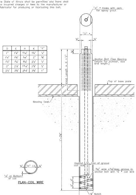
MATERIALS FOR ILLINOIS COIL-LOCK ANCHOR BOLT
