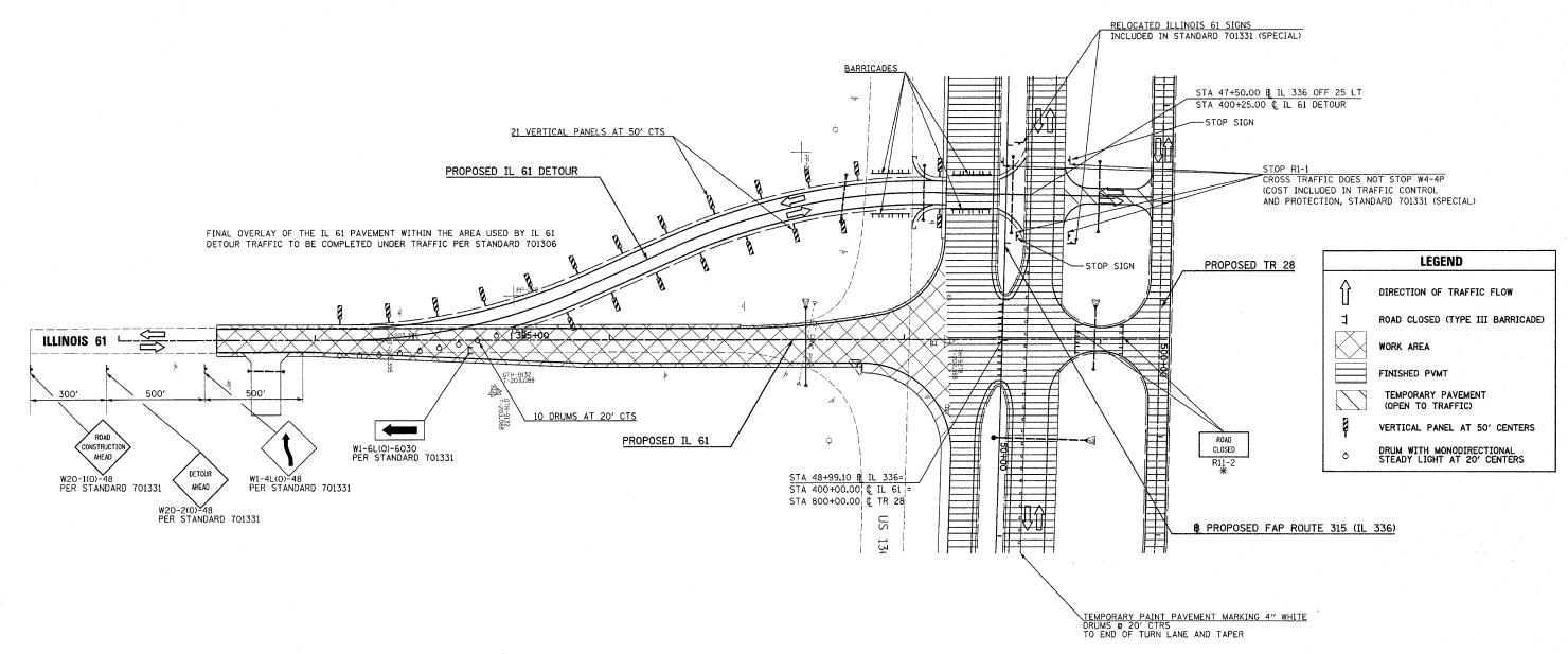
TRAFFIC CONTROL FOR THE IL 61 DETOUR SHALL BE PER THIS DETAIL AND THE APPLICABLE PORTIONS OF STD 701331, TRAFFIC CONTROL TO BE PAID FOR PER EACH AS TRAFFIC CONTROL AND PROTECTION, STANDARD 701331 (SPECIAL)
