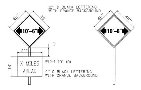
THE CONTRACTOR SHALL BE RESPONSIBLE FOR FUNISHING, ERECTING AND MAINTAINING THESE SIGNS.TO BE POST MOUNTED. A TOTAL OF THREE SIGNS NEEDED- 2 ON US 41 IN INDIANA ( ONE NB AND ONE SB LANE JUST NORTH OF INDIANA 10). PLACE THE OTHER SIGN ON INDIANA 10.
