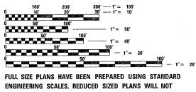
CONFORM TO STANDARD SCALES. IN MAKING MEASUREMENTS ON REDUCED PLANS, THE ABOVE SCALES MAY BE USED.
