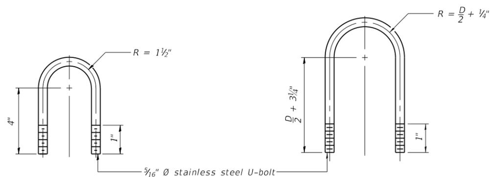
**DAMPING DEVICE MOUNTING TUBE U-BOLT DETAIL**
