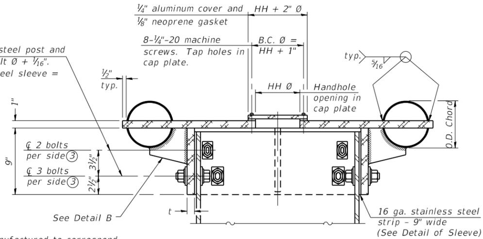
④ Collar I.D. shall be manufactured to correspond to O.D. of actual galvanized post and stainless steel sleeve plus  $1/8"$  ( $\pm 1/16"$ ). Maximum gap between post and collar at any location equals  $1/8"$  before tightening bolts.
