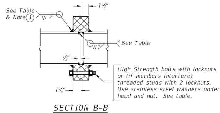
① Splicing Flanges shall be attached to each truss unit with the truss shop assembled to camber shown. Truss units shall be in proper alignment and flange surfaces shall be shop bolted into full contact before welding. Sufficient external welds or tacks shall be made to secure flanges until remaining welds are made after disassembly. Adjacent flanges shall be "match marked" to insure proper field assembly.
