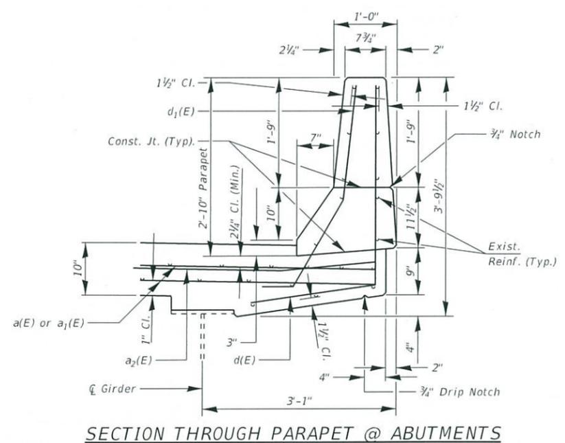
**SECTION THROUGH PARAPET @ ABUTMENTS**
