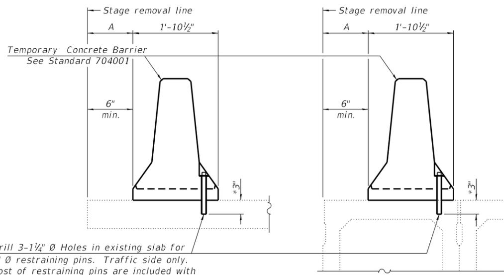
Drill 3-1/4" Ø Holes in existing slab for 1" Ø restraining pins. Traffic side only. Cost of restraining pins are included with Temporary Concrete Barrier. No restraint is required when "A" is greater than 3'-1".
