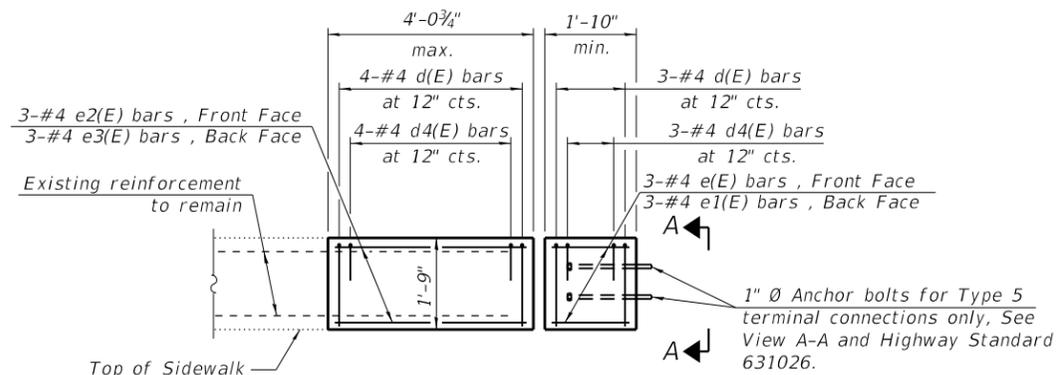
**Inside Elevation - West Parapet**
