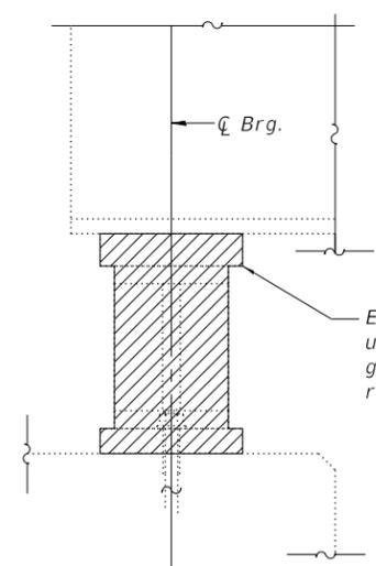
**EXISTING BEARING REMOVAL DETAIL**
