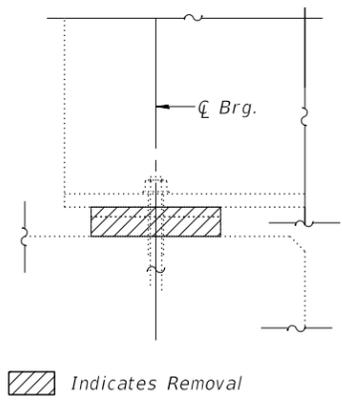
**EXISTING BEARING REMOVAL DETAIL**
