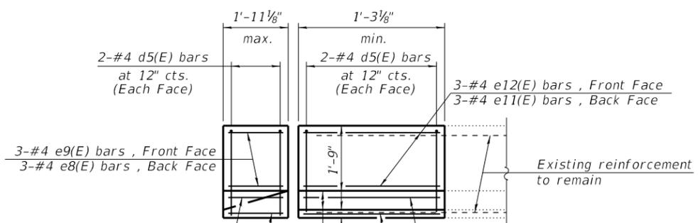
**Inside Elevation - East Parapet**
