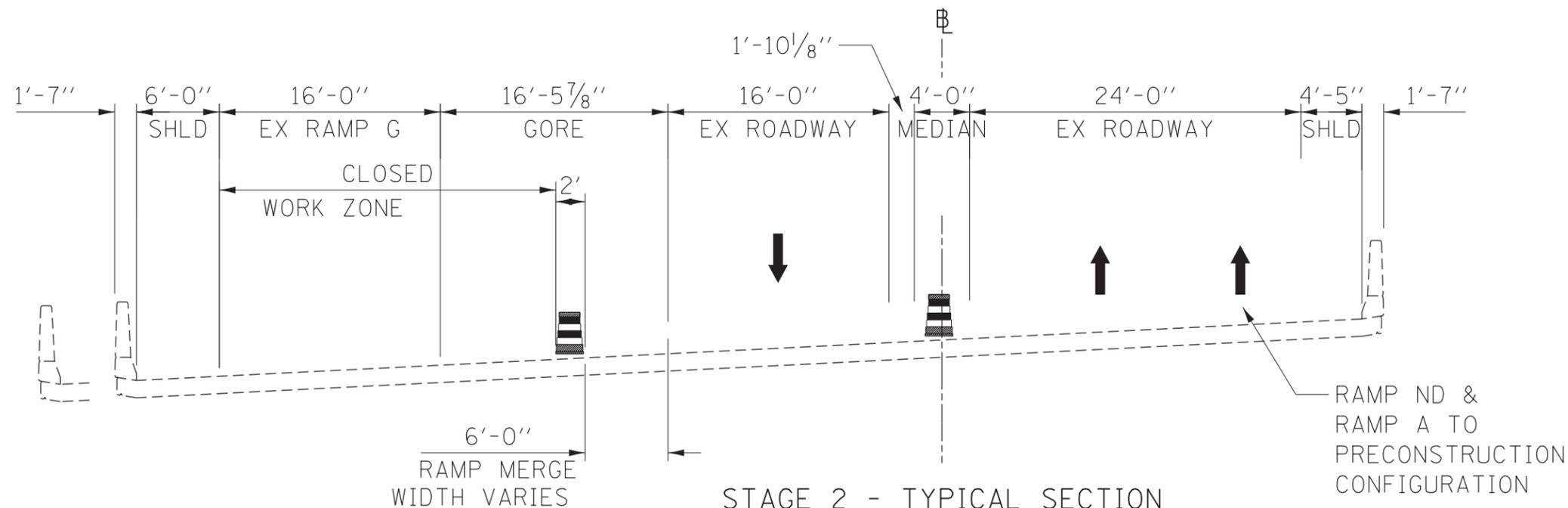
STAGE 2 - TYPICAL SECTION RIVERFRONT DRIVE SPUR
