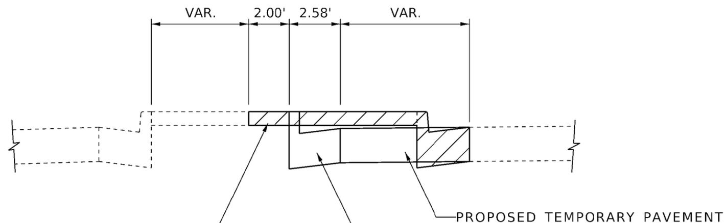
VOID SHALL BE FILLED WITH COMPACTED CA 6. THIS WORK SHALL BE INCLUDED IN THE COST OF THE PROPOSED CURB AND GUTTER.
