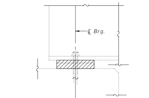
EXISTING BEARING REMOVAL DETAIL
