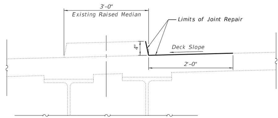
**MEDIAN JOINT REPAIR DETAIL**
