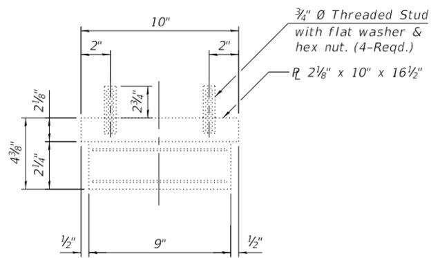
**EXISTING BEARING ASSEMBLY AT NORTH ABUTMENT**
