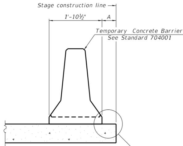
When "A" is 3'-1" or less, the temporary concrete barrier shall be restrained to the new slab according to Detail I, II or III. No restraint is required when "A" is greater than 3'-1".
