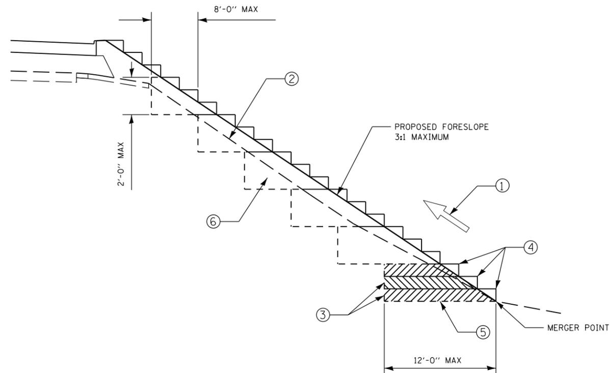
**TYPICAL BENCHING FOR EMBANKMENT DETAIL**
