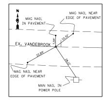
VANDEBROOK ACCESS RD. P.O.T. STA. 95+03.29 MAG NAIL IN PAVEMENT 597,358.8250 N 2,301,452.6700 E
