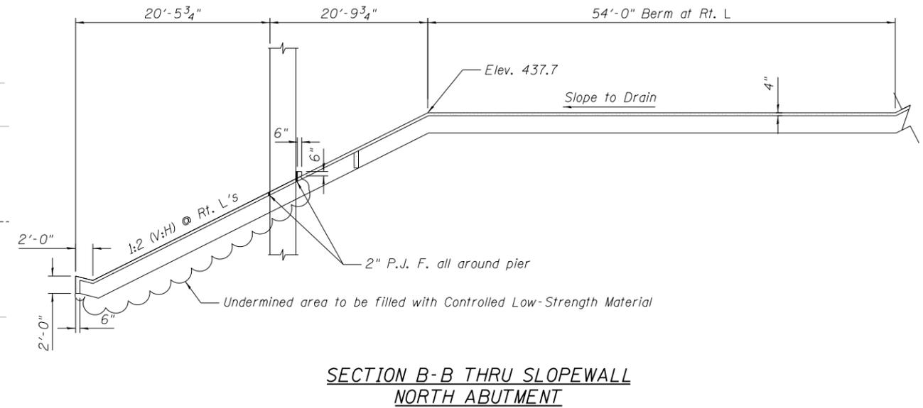
SECTION B-B THRU SLOPEWALL NORTH ABUTMENT
