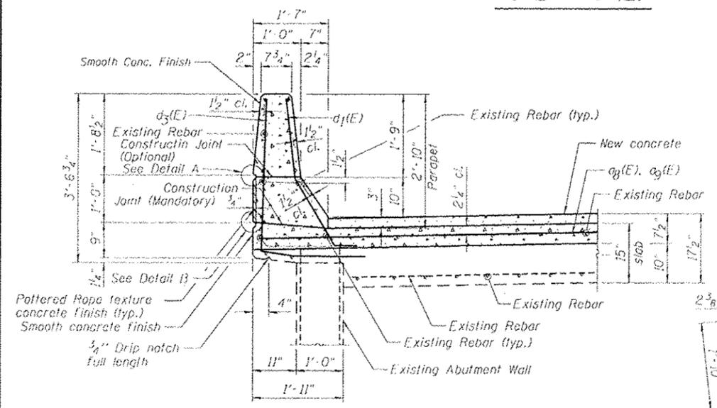
**SECTION C-C THRU ABUTMENT PARAPET**
