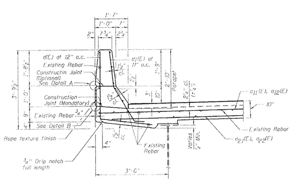
SECTION D-D THRU BRIDGE PARAPET
