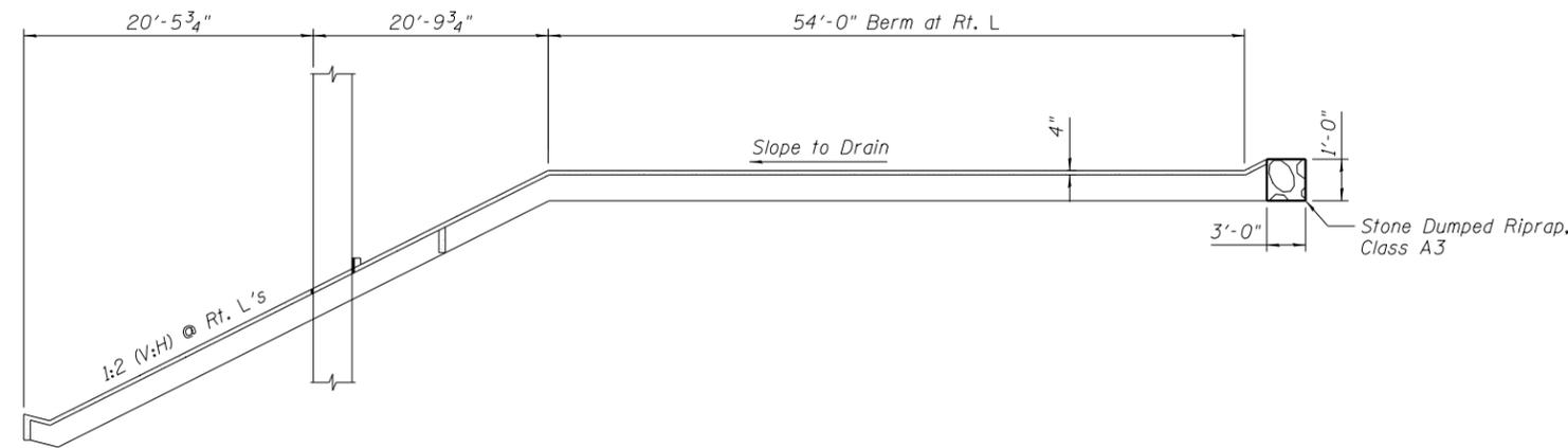
SECTION C-C THRU SLOPEWALL NORTH ABUTMENT
