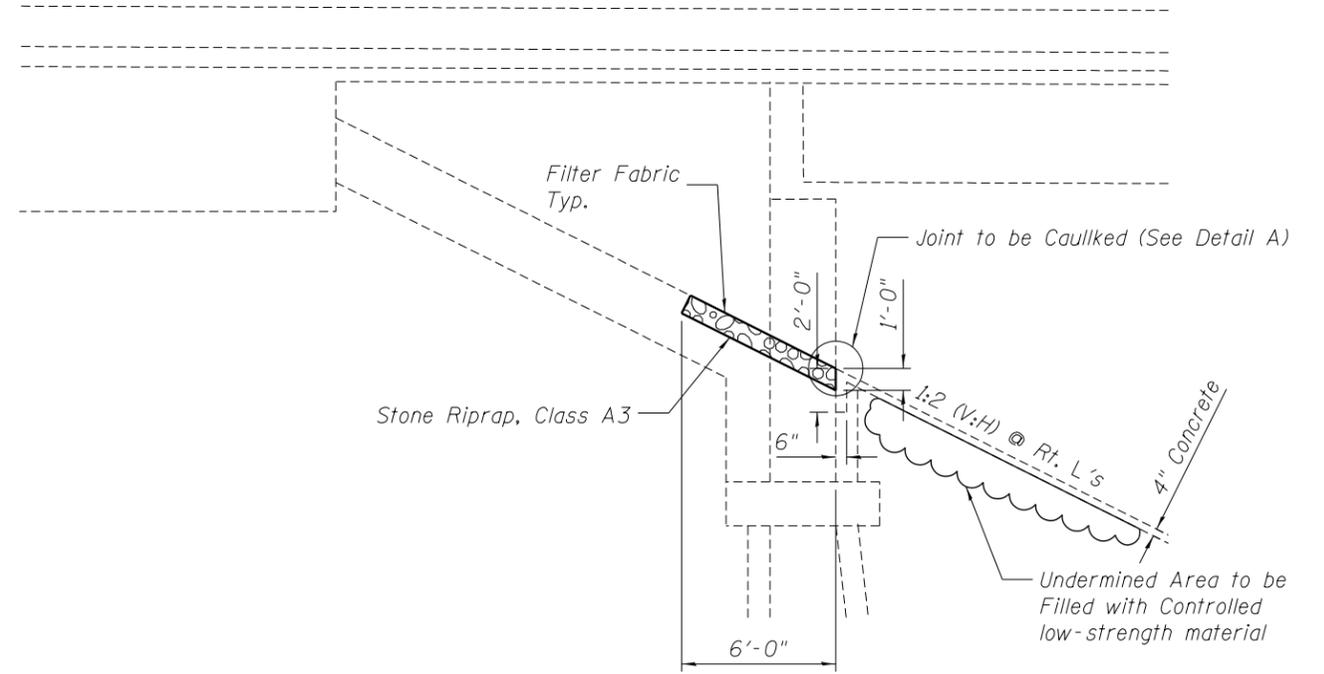
SECTION A-A THROUGH SLOPE WALL
