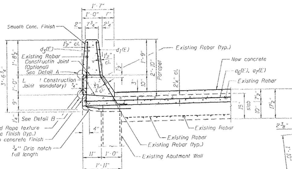
SECTION C-C THRU ABUTMENT PARAPET
