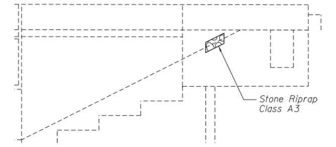
**RIPRAP PLACEMENT ON SLOPE**
