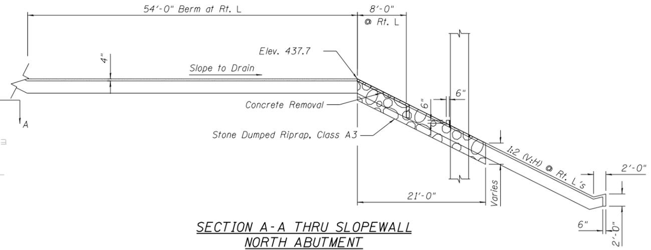
SECTION A-A THRU SLOPEWALL NORTH ABUTMENT
