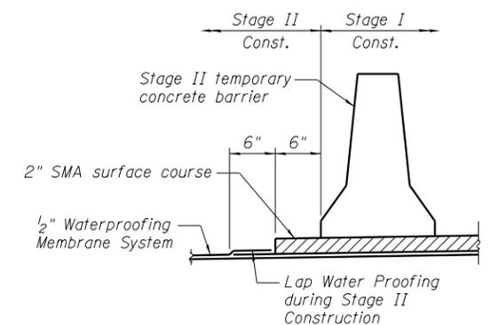
**WATERPROOFING STAGING TYPICAL DETAIL**
