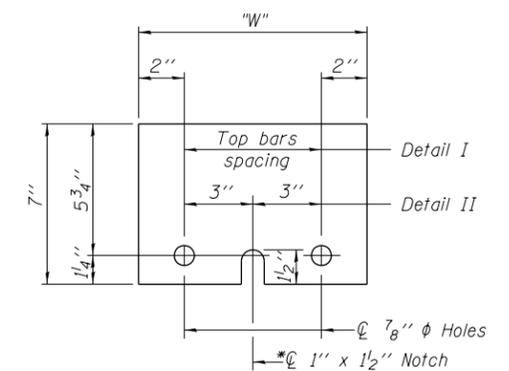
**STEEL RETAINER  $\bar{L}$  1" x 7" x "W"**
