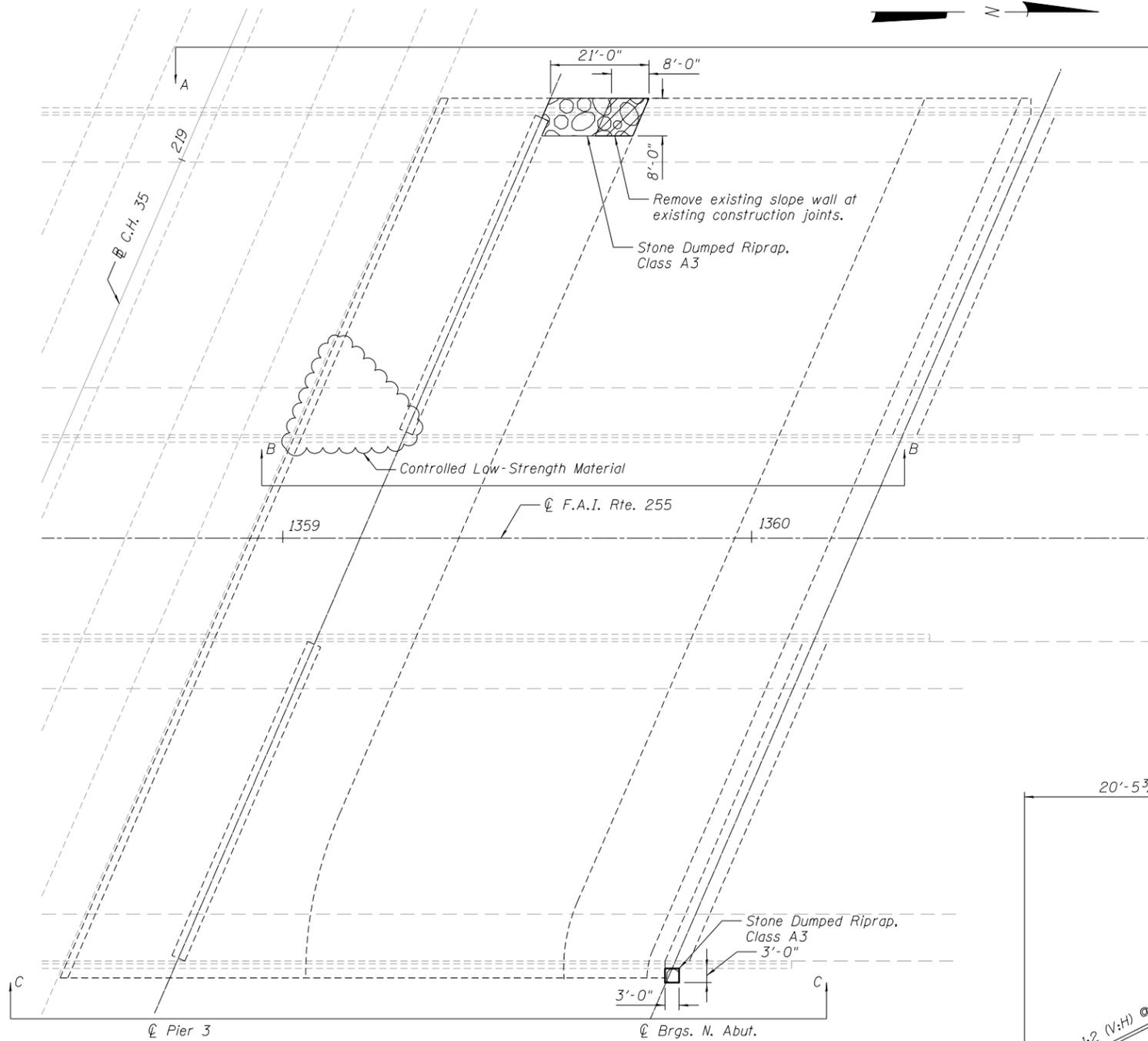
PLAN OF SLOPEWALL NORTH ABUTMENT
