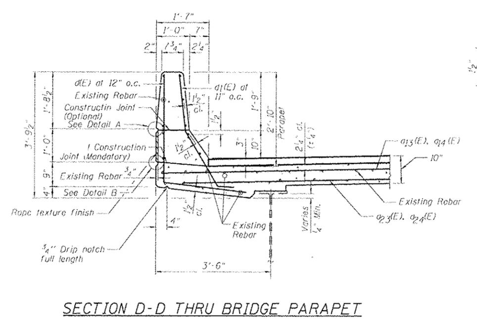
**SECTION D-D THRU BRIDGE PARAPET**
