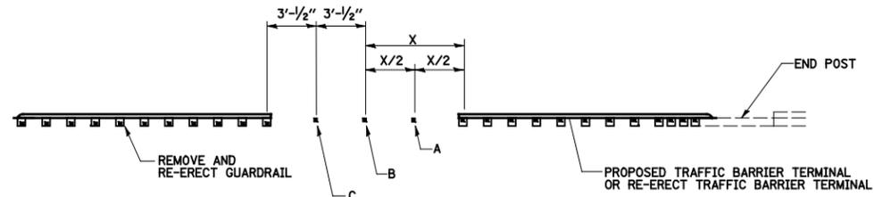
**DETAIL OF TRAFFIC BARRIER TERMINAL CONNECTION TO PROPOSED GUARDRAIL SPLICE**
