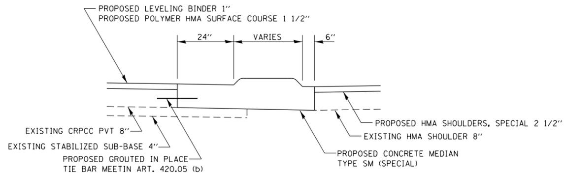
CONCRETE MEDIAN TYPE SM (SPECIAL) SECTION
