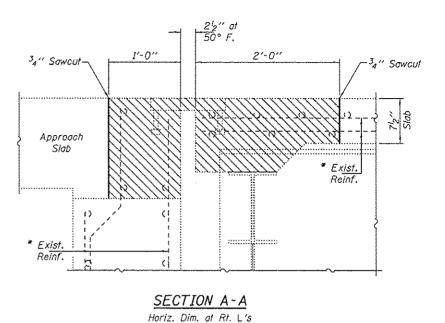
\* Existing reinforcement bars extending into the removal area shall be cleaned, straightened and incorporated into the new construction. Any reinforcement bars that are damaged during concrete removal shall be replaced with an approved bar splicer or anchorage system. Cost included with Concrete Removal.
