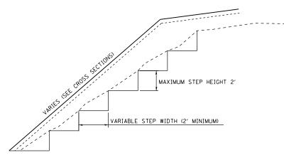
NOTE: THIS DETAIL SHALL BE APPLIED TO SIDESLOPE FILLS WHERE THE EXISTING SLOPE IS STEEPER THAN 1:3.
