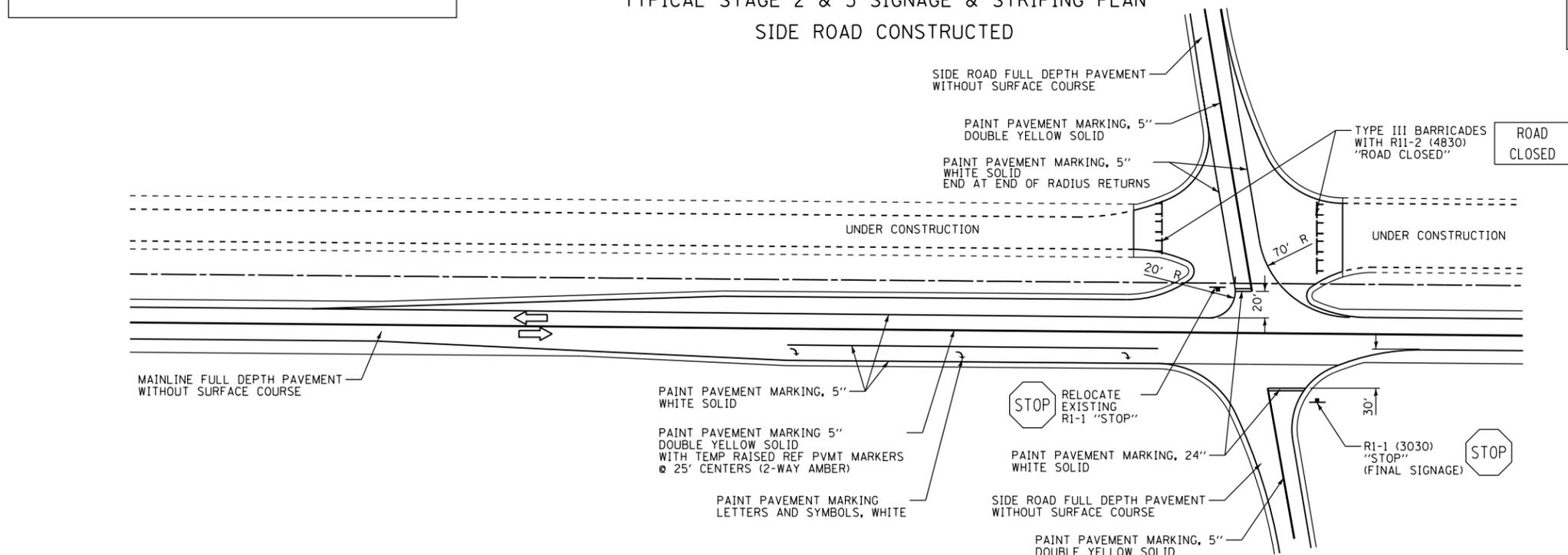
SEE SIGNING & STRIPING PLAN SHEETS FOR STRIPING ON TOP LIFT OF FULL-DEPTH PAVEMENT.
