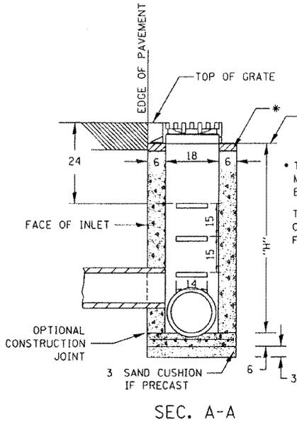
• THE WALL ADJUSTMENTS SHALL BE MADE WITH CONCRETE BUILDING BRICK OR CLASS SI CONCRETE.
