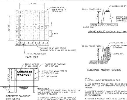
2. HARDENED CONCRETE CAN BE PROPERLY RECYCLED AND REUSED CHSITE OR HAULED OFF-SITE TO AN APPROPRIATE FACILITY.
