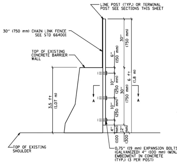
FENCE ATTACHED TO BACK OF EXISTING WALL - SECTION
