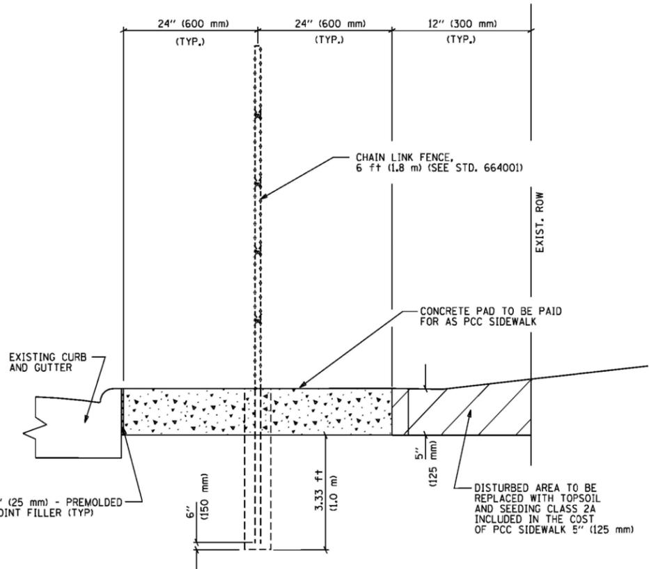
FENCE MOUNTED ON CONCRETE PAD - SECTION
