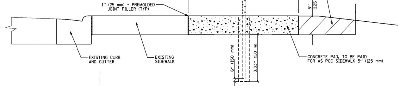
FENCE MOUNTED ON CONCRETE PAD ALONG EXISTING SIDEWALK - SECTION
