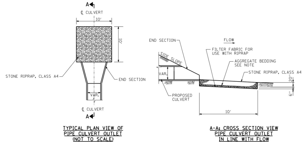
NOTE: AGGREGATE BEDDING SHALL BE INCLUDED IN THE COST OF STONE RIPRAP, CLASS A4
