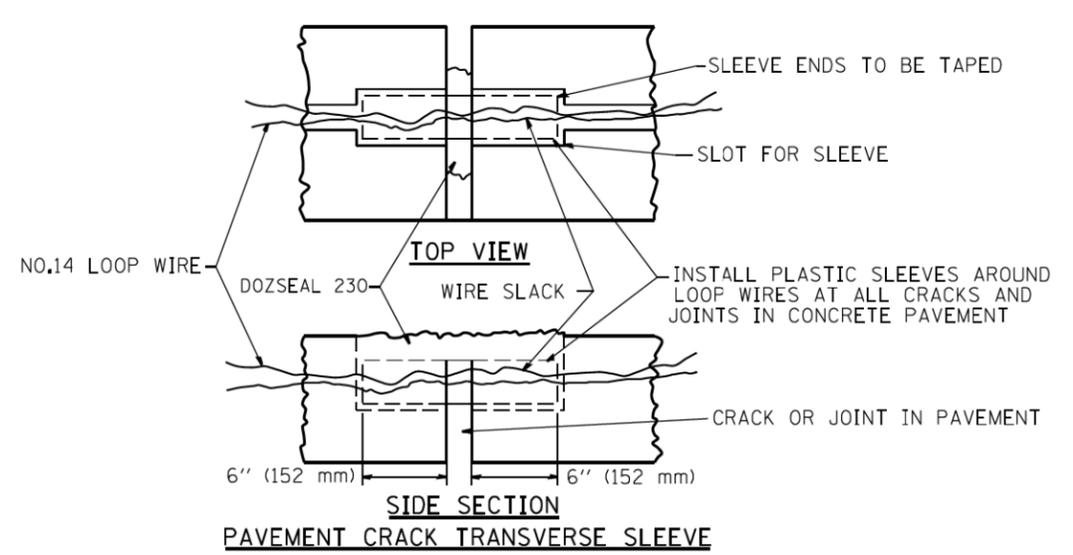
**PAVEMENT CRACK TRANSVERSE SLEEVE**
