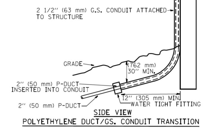
**POLYETHYLENE DUCT/GS. CONDUIT TRANSITION**
