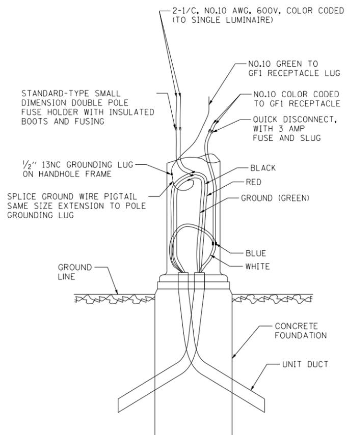
**POLE BASE WIRING DETAIL
