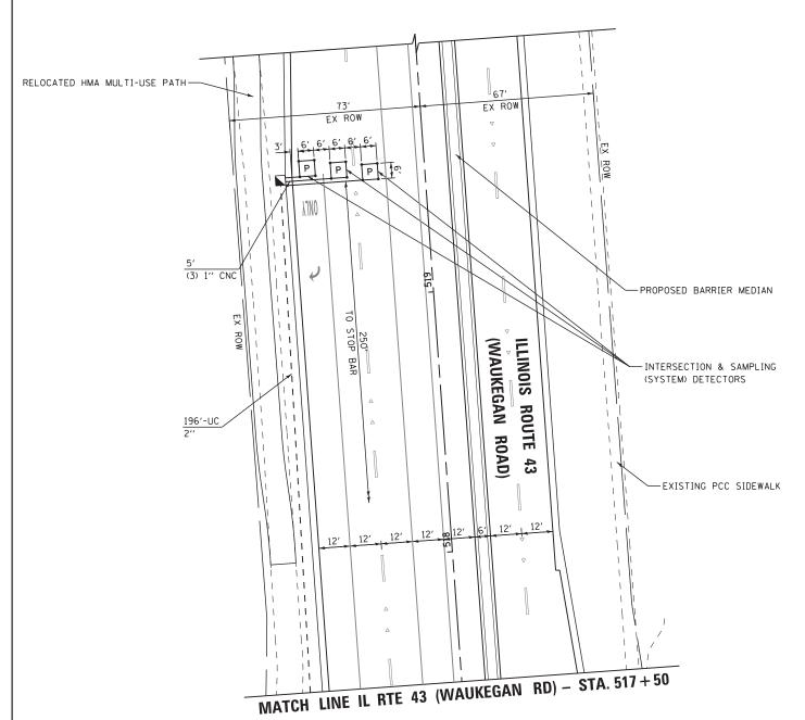
ALL LOOPS SHALL BE PREFORMED WITHIN LIMITS OF RECONSTRUCTION
