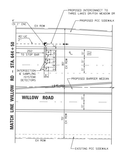
ALL LOOPS SHALL BE PREFORMED WITHIN LIMITS OF RECONSTRUCTION
