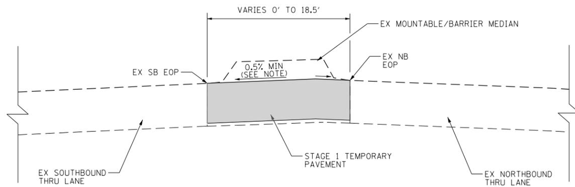
STAGE 1 TEMPORARY PAVEMENT TYPICAL SECTION AT MEDIAN
