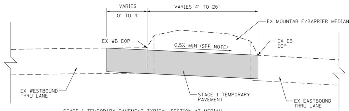
STAGE 1 TEMPORARY PAVEMENT TYPICAL SECTION AT MEDIAN
