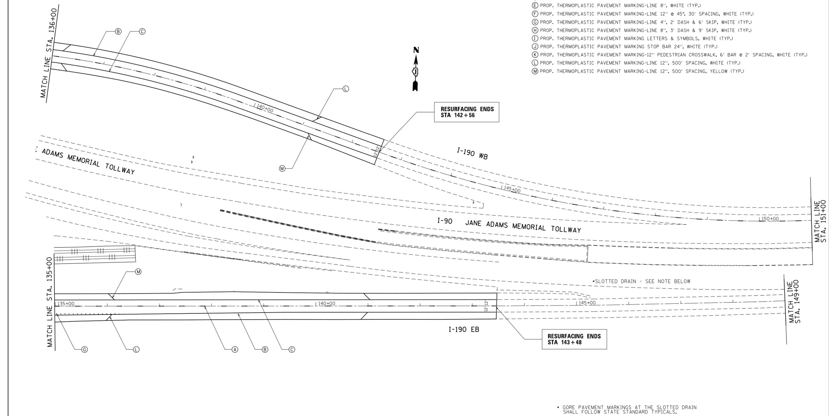
\* GORE PAVEMENT MARKINGS AT THE SLOTTED DRAIN SHALL FOLLOW STATE STANDARD TYPICALS.
