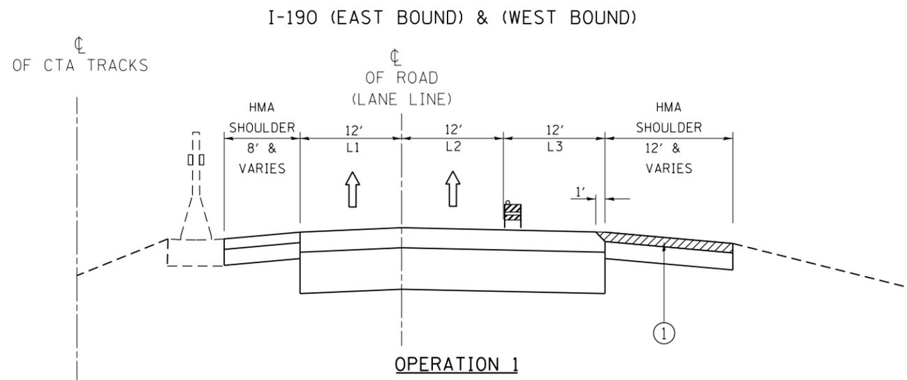
① HOT MIX ASPHALT SURFACE REMOVAL, 3 3/4"
