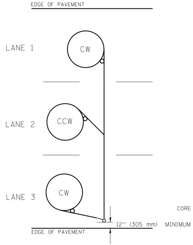
TYPICAL 6' (1.83 m) DIA. INDUCTION LOOP CORE DRILL
