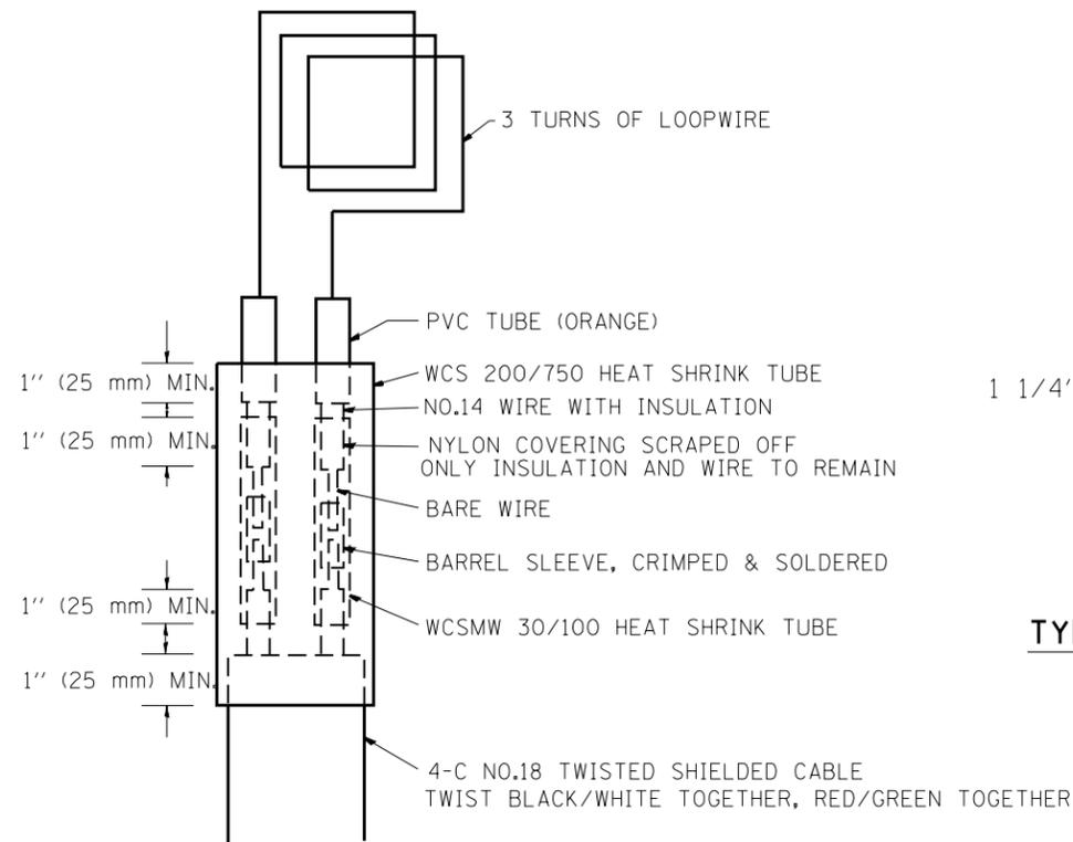
MINIMUM 1" (25 mm) HEAT SHRINK TUBING OVERLAP ON WIRE, PVC & SHIELDED CABLE TO FORM WATER TIGHT SEAL
