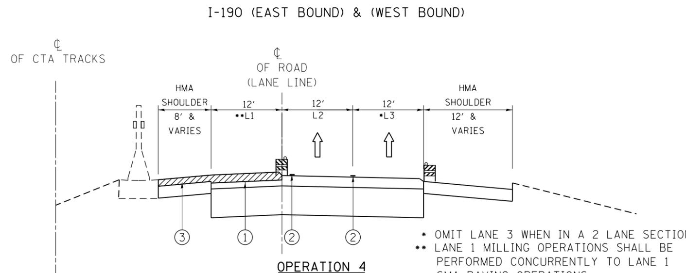
① HOT MIX ASPHALT SURFACE REMOVAL, 4"
