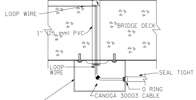
JUNCTION BOX, STAINLESS STEEL ATTACHED TO STRUCTURE
