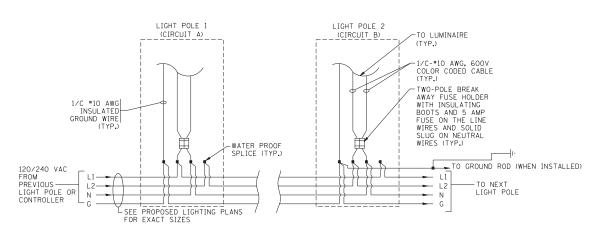
LIGHT POLE WIRING DETAIL
