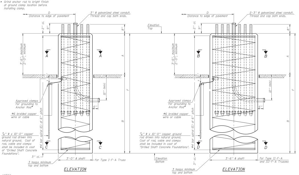
FOUNDATION DESIGN TABLE Maximum Maximum "B" Anchor Rods Shaft Anchor Rod Post Base Truss Total Sign Area CantileverLength Depth Diameter Diameter Circle Diameter Туре Sheet No. (sq ft) (ft) (ft)(in) (in) (in) 17′-6′ 22 I-F-A 0SF-A-4 25 200 3.0 22'-0' II-F-A OSF-A-5 30 400 3.5 12 400 0SF-A-5 24'-0'
