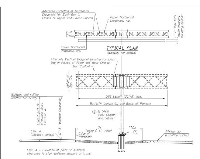
\*\* Elevation A2 and dimension D2 not used when butterfly structure is mounted on right side of the shoulder.
