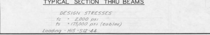
TYPICAL SECTION THRU BEAMS
