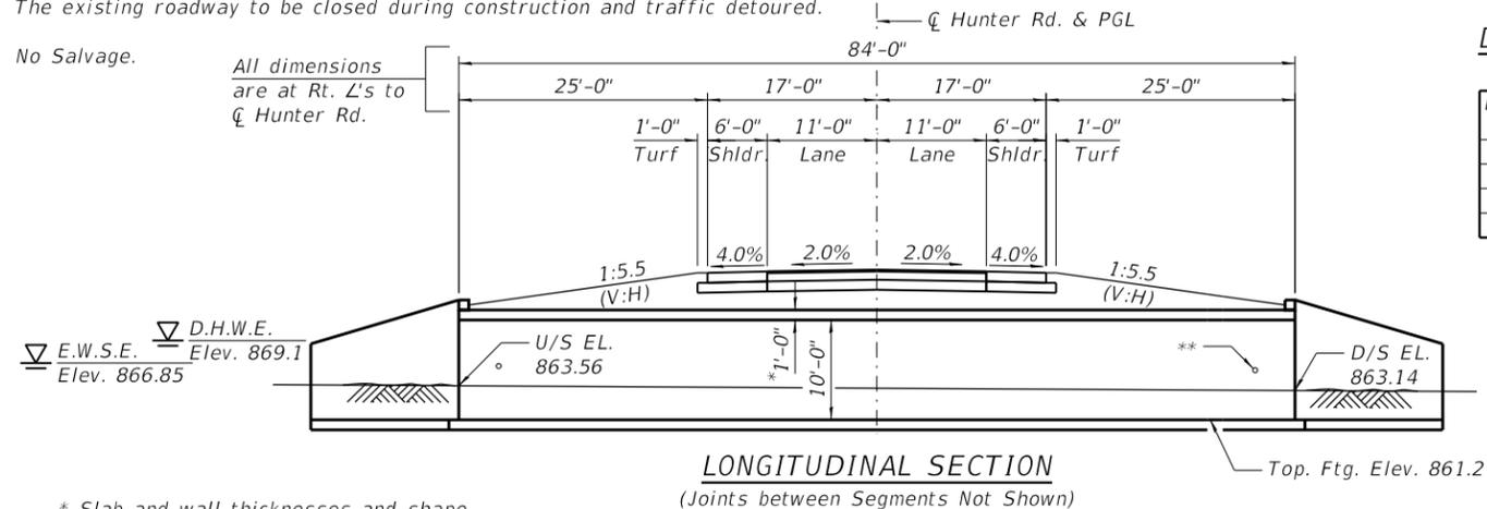
\* Slab and wall thicknesses and shape may vary as per manufacturer's design.
