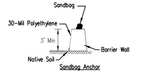
**BARRIER WALL ANCHOR SECTION**
