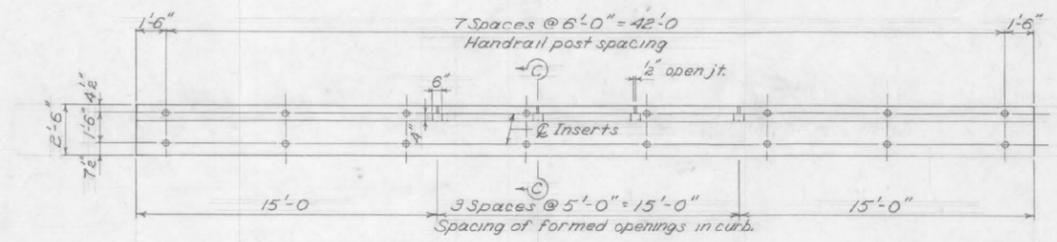
ELEVATION OF OUTSIDE BEAMS
