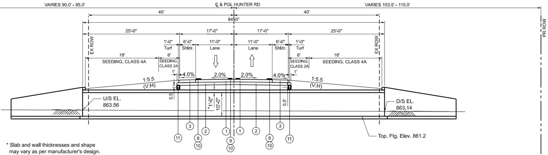
**PROPOSED TYPICAL SECTION AT THREE-SIDE STRUCTURE**
