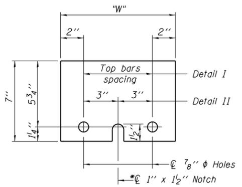
**STEEL RETAINER  $\bar{L}$  1" x 7" x "W"**
