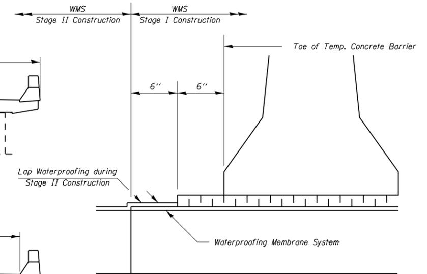
**Waterproofing Treatment at Stage Construction**
