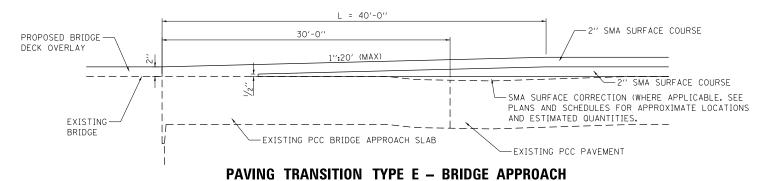
SMA ON EXISTING PCC BRIDGE APPROACH SLAB AND PAVEMENT (WITH BRIDGE OVERLAY)
