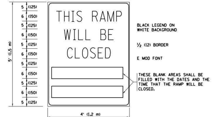
THESE SIGNS ARE REQUIRED ON BOTH SIDES OF THE RAMP, MINIMUM OF 1 WEEK IN ADVANCE OF THE CLOSURE.
