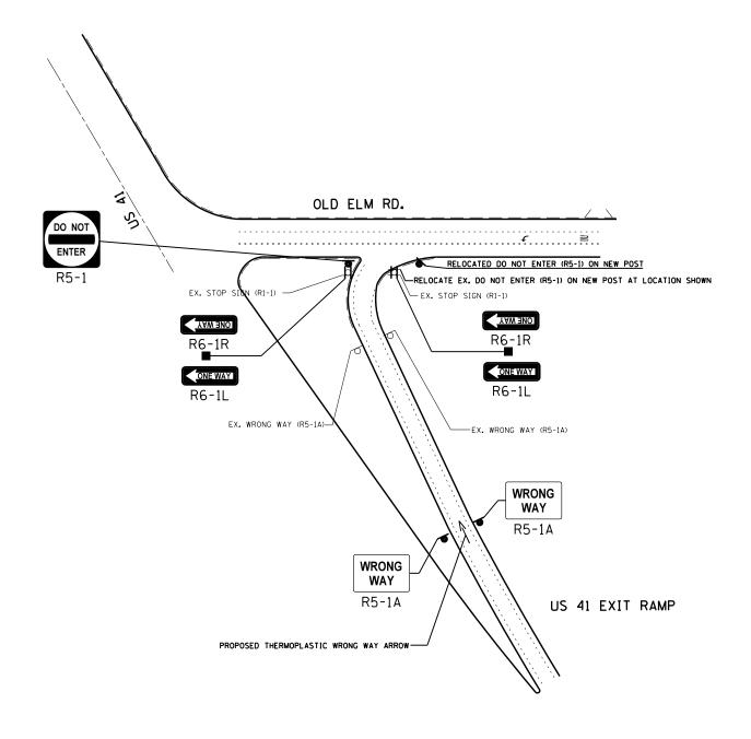
NOTE: SIGN ASSEMBLIES GREATER THAN 16 SQUARE FEET REQUIRE 2 TELESCOPING STEEL SIGN SUPPORTS.
