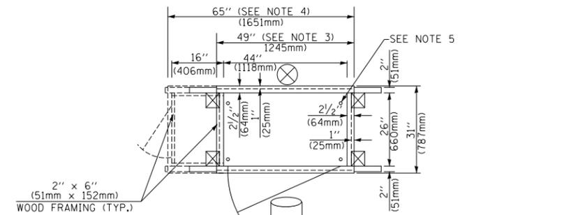
TEMPORARY SIGNAL CONTROLLER WOOD SUPPORT PLATFORM
